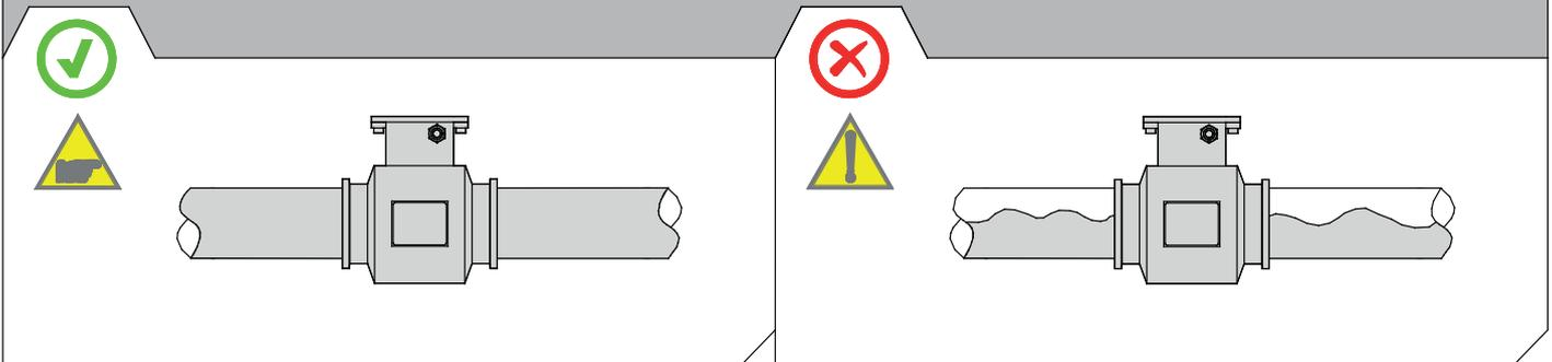
Install the sensor away from bends and hydraulic accessories
